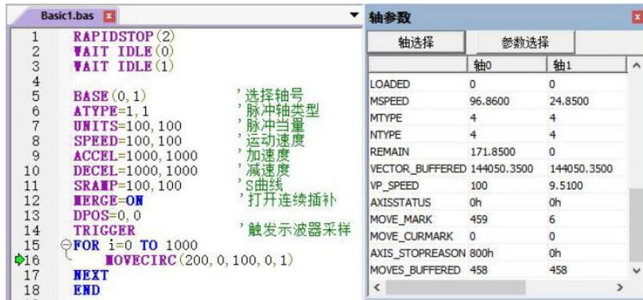
Motion Buffer Block Effect – Circular Interpolation
